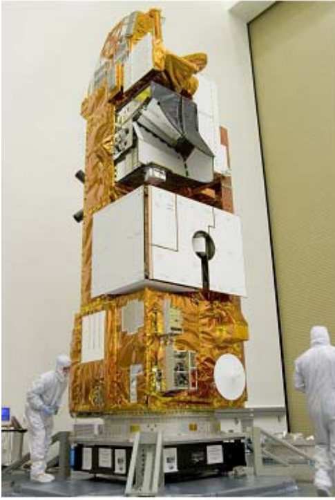
This is the Aura satellite before being launched. It is folded so it can fit into the launch rocket.
